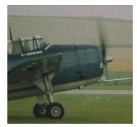
This Avenger, which is beginning its take off at Duxford, does not show any airfield weathering, 'though it does show how it can happen. If you look closely below the cowl (grey streaks against grass), you can see vortices of moisture sucked out of the damp atmosphere and also pulled up from the grass.
