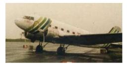
This DC-3 stood outside for over a year at Newcastle without any maintenance except periodic engine runs. Dirt has gathered in all the panel lines showing most clearly around the nose and engine cowlings.
