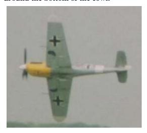
This slightly grainy picture of a Bf 109J shows streaks of blackened oil, from the oil cooler vent in the bottom of the cowl, extending back along the fuselage
