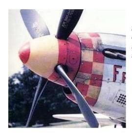
Several replacement fasteners can be seen on this Mustang engine cowling as a result of wear from the constant removal and replacement of the panels by the ground crews. Paint has also chipped away along panel edges.
