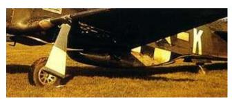
This P-51 shows severe paint damage on the radiator scoop as a result of dirt and dust being blasted back by the prop.
