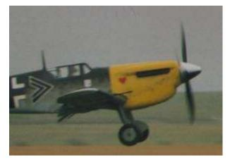
This Bf 109J shows signs of fretting along the yellow cowl panels. The dark fuzzy stains extend back from the lower cowl panel fasteners.
