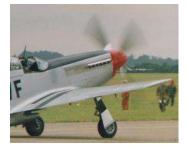
The metal panel around the exhaust stacks is steel and as a result, it discolours in a different way to aluminium. This airplane is actually painted silver rather than being natural metal, but on a natural metal airplane, the aluminium dulls down while the steel does stain. On olive drab painted airplanes, the paint fades differing amounts on steel and aluminium parts.
