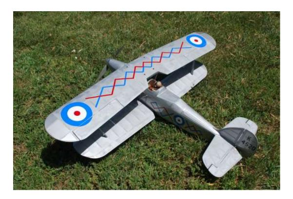
Span 46 inches, All up weight 3.6 lb Motor Prop Drive 3542 1000KV Prop 11x5.5 APC Battery Turnigy 3 cell 3000 mAh ESC Turnigy Plush 40 amp As can be seen from the plan the Gordon Whitehead construction details are that close to the full size plane a bit too complicated for me, so I simplified the construction using methods I have used for years, a proper d-box structure for the wings.
