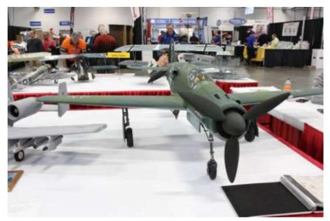
The twin is 1/6-scale and took 2 1/2 years to complete. The Do 335 is finished with Latex house paint and includes functional flaps, homemade pneumatic retracts and navigation lights
