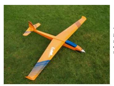
The orange model is called Firestreak and is 72 inch span, foam core wing, 2.2lbs weight and has a motor giving 750 watts. It is intended as an entry level model for F5B competition although I think that it will be only used for fast aerobatics.
