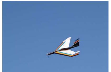
The wing with the black fuselage is the Italda and is a 95 inch foam core wing, 10 sq feet area, .6 oz glass cloth/varnish covering, balsa fuse. Weight is 85 ozs. Motor is of 200 watts. Designed as a sailplane. (no aerobatics). Controls are elevons and speed brake/lift flap.
