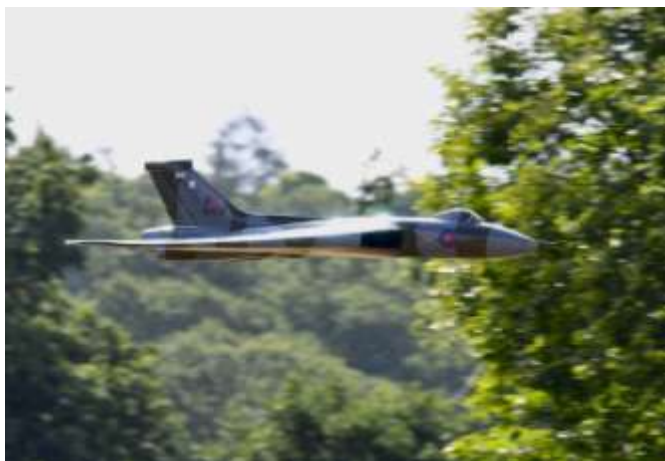
Large Avro Vulcan form the Tony Nijhus plan, 14 cells, Schubler fan, sounded just light a turbine
