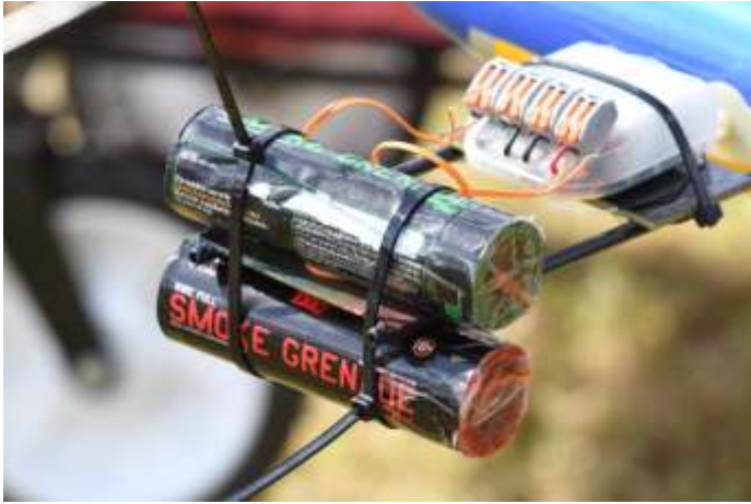
Smoke system on wingtip of large scale glider, turbine powered of course
