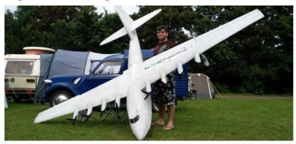
Built and flown by Jürgen Schönle, this eight-motor model has over a 13-foot wingspan yet weighs just under 11 pounds, thanks to its foam and carbon-fiber construction. The 1/22-scale aircraft is powered by a single 3S, 4000mAh LiPo! Jurgen spent only a month building this model. Howard Hughes would be proud! Thanks to RC Media World for taking this video at the seaplane event in Edersee, Germany earlier June 2017.
