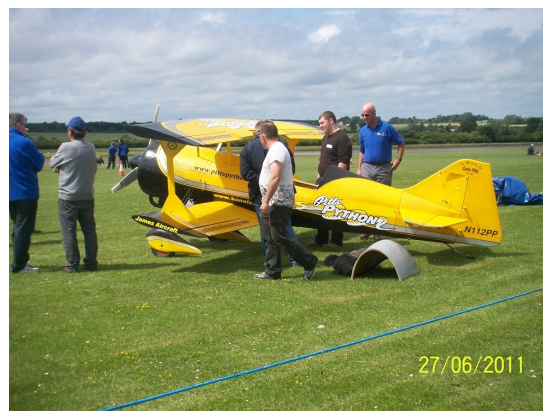
The large model shown is about 3/4 full size Pitts special , powered by a 250 cc Hirth two stroke
