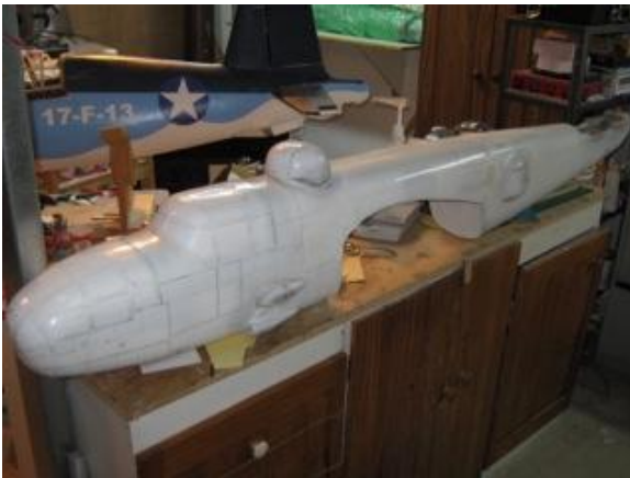
A plug for B25 to make fibreglass mold
