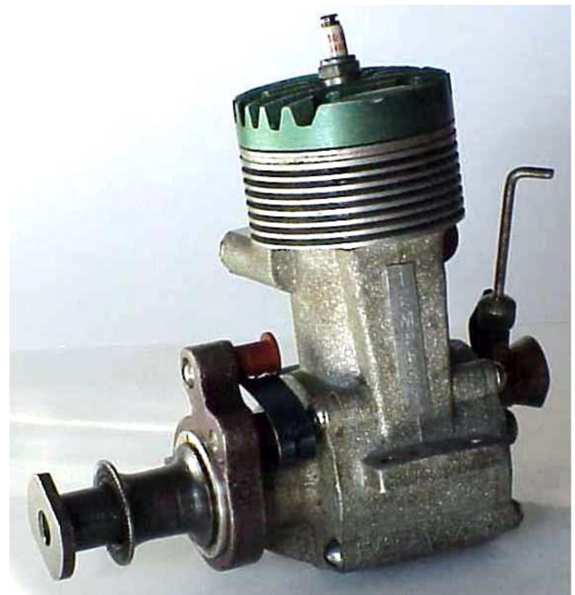
Tempest 60 shown with spark ignition, most were used on glow.
