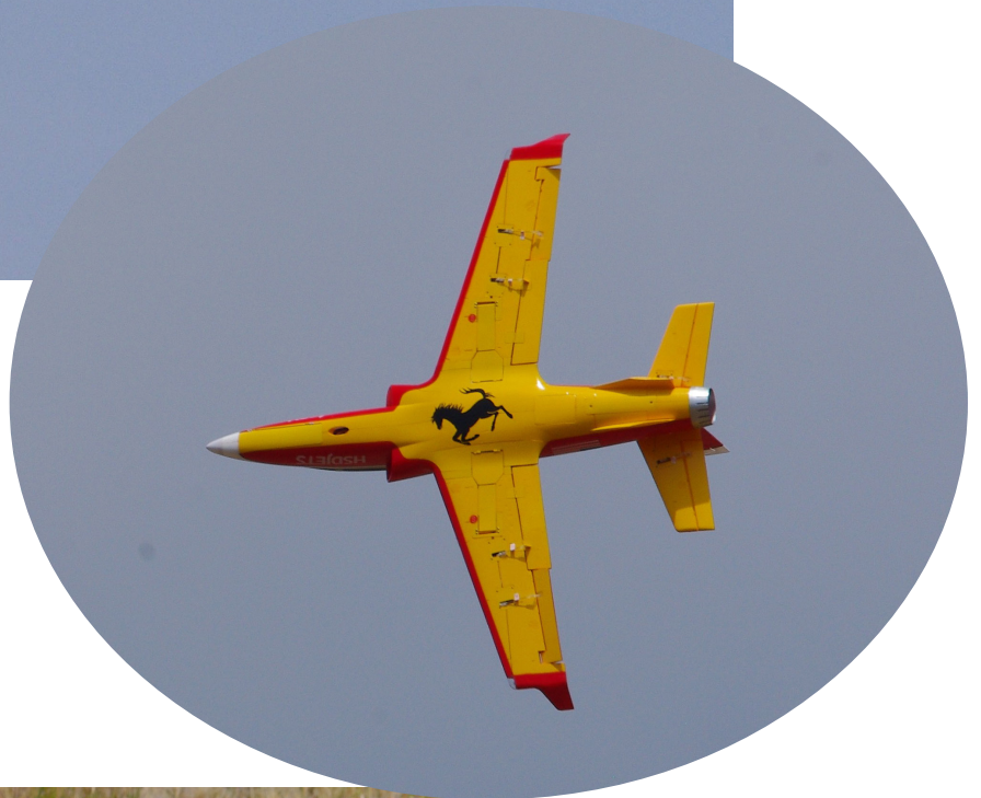
Damian Blackwell's new Viper: A larger and updated version of his earlier models. Note the curved upturned wing tips. Upgraded fan rotor as well.
