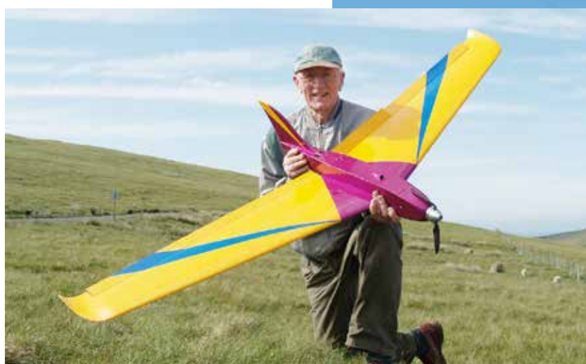
Flying wing with me. This is the Gulp, 82 inch span, all built up construction. Nicely aerobatic.
