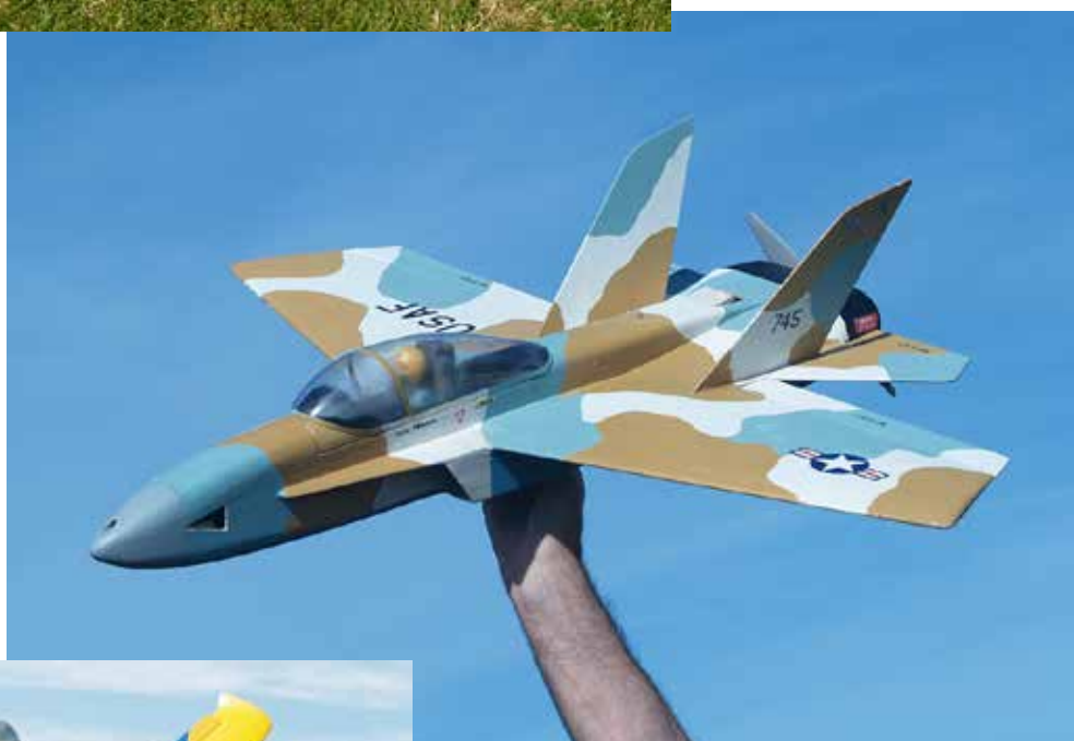
Dominator 36. 36 inch span all wood with a sheet wing. This is the single motor version and there is another twin version. These have not been offered to the magazine as there is also a 42 inch version which they prefer, the plan of which is on its way to being finished.
