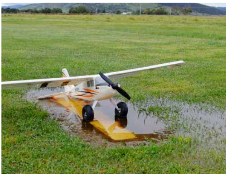
Peter Ralph's Timber UMX Ultra Micro. The runway being chronically water logged, STOL models both large and small have proved most practical. Conventional models have in some cases been unable to take off, and if they do become airborne, will quite often tip onto their nose on landing due to the extremely high drag of the grass with a layer of water on the ground surface.
