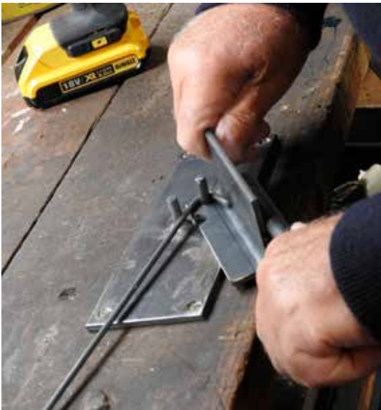
L: Chris's handmade heavy wire bender fixed to the bench.
