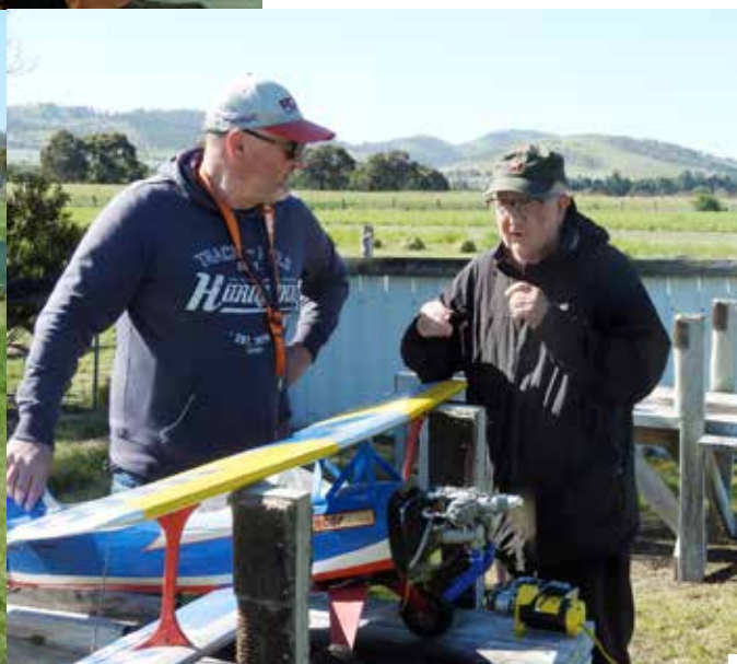
Jon Hall and Damian Blackwell discussing Peter Ralph's Seagull brand Skybolt powered by a 21cc twin cylinder petrol engine.
